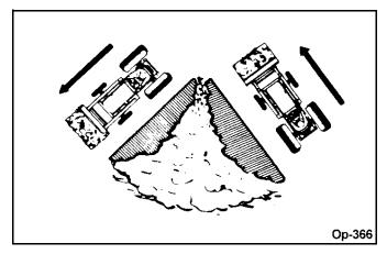
If the pile sides are too high and liable to cause cave-in, use loader to break down the sides until a slot can be cut over the top.
